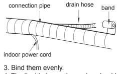
4. The liquid pipe and gas pipe should be bound separately at the end.
