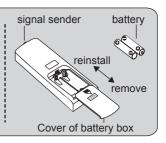
3. Reinstall the cover of battery box.
